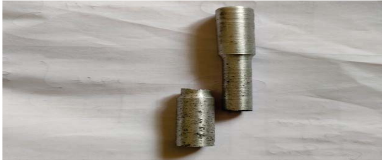
FIGURE 8. Specimen after undergoing tensile load
