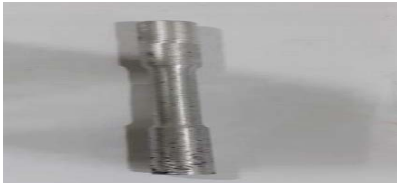
FIGURE 7. Specimen prepared for tensile test
